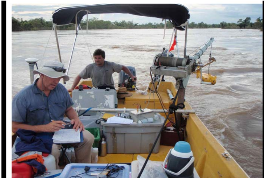
2009 trip down the flooded Mitchell River measuring suspended sediment concentration and bedload transport (photo courtesy of Jeff Shellberg).
